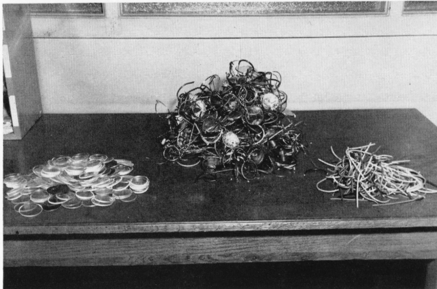
In keeping books on the human machine, people know the debit side of their ledger — a missing eye or limb is self evident. But the credit side is skipped in many cases where eyes or limbs were saved through proper use of safety equipment. The above safety spectacles were used in a certain period in Scovill. The numerous broken lenses testify how they stopped flying fragments, splashes of molten metal. They'll save your eyes, too!
